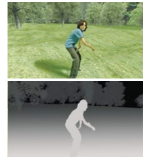
Figure 2: The 2D-plus-depth format is used as the 3D video format in our 3D display systems. (Top) A conventional 2D image providing 2D compatibility and 3D texture information. (Bottom) Depth map providing 3D geometry information by depth-per-pixel.
