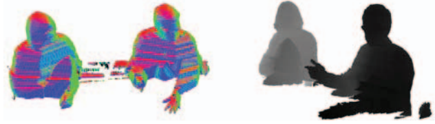
Fig. 3. left) Example for a reconstructed volume for a voxel size of 5^3\text{mm} . Nine cameras were used, right) depth map generated from the reconstructed volume using the SfS algorithm
