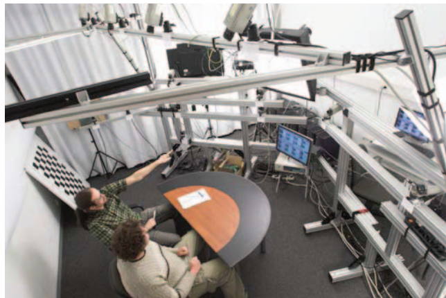
Fig. 5. Experimental setup for combined Visual Hull and HRM based analysis system in the context of 3D video conferencing
